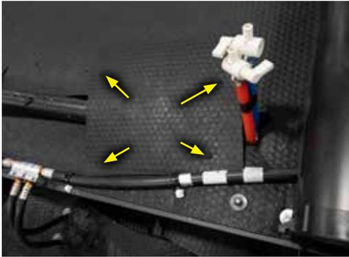
Strategically positioned, our multiple access points allow easy entry to the undercarriage. Using only 4 screws, this removable panel provides a convenient way to help inspect and maintain the RV systems.
