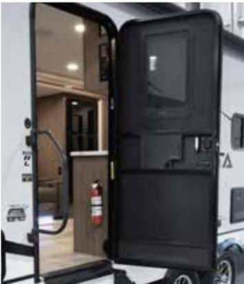
The integrated friction hinge door will hold the door open in any position. Our hinge torque also prevents the door from slamming open or closed, and keeps the door steady in winds up to 15 mph!
