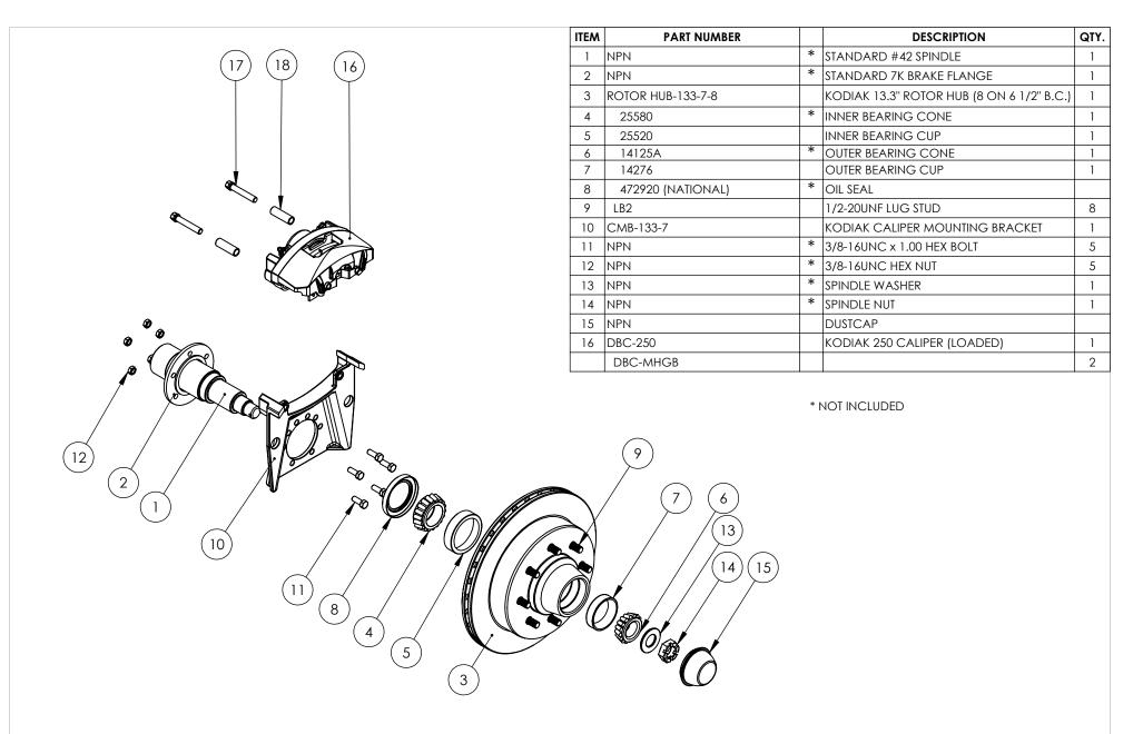
NOTE: On air ride suspensions, Kodiak recommends "clocking" calipers as close to the lowest amplitude point as possible on the wheel end assembly.
